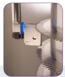
Housed in thermally efficient stainless steel canisters, the sample first undergoes a precise controlled rate freeze (CRF).
